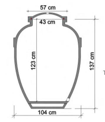
Tall:133 cm/52,4 inch Max diameter: 104 cm/41 inch Weight: 250kg/550 pounds Ceramic with programmed porosity Ceramic thickness: 25 mm/1 inch Inside and outside hand sanded Ceramic cap with rubber ring Bubble hole 45 mm/1,77 inch Inox and bronze closing system Quick release cap Total out put Din 40–50–Macon Triclamp.
