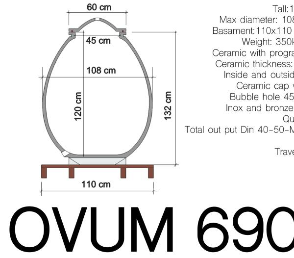
Tall: 150 cm/59 inch Max diameter: 108 cm/42,5 inch Basament: 110x110 cm/43,30 inch Weight: 350kg/770 pounds Ceramic with programmed porosity Ceramic thickness: 25 mm/1 inch Inside and outside hand sanded Ceramic cap with rubber ring Bubble hole 45 mm/1,77 inch Inox and bronze closing system Quick release cap Total out put Din 40-50-Macon Triclamp. Oak pallet Travertine basement
